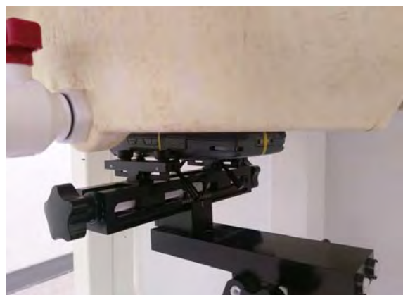
Fig.16 EUT Front side to flat phantom
