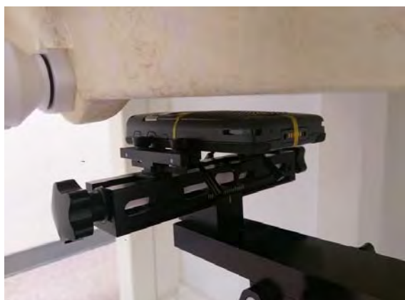
Fig.8 EUT Back side to flat phantom
