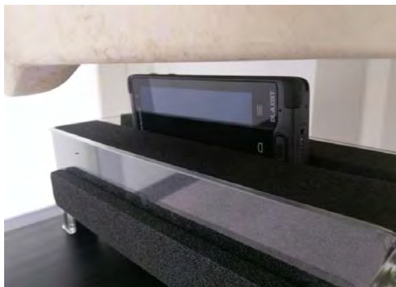
Fig.13 EUT Right side to flat phantom
