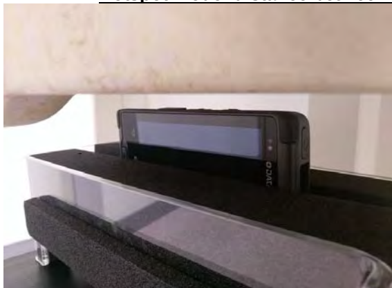
Fig.12 EUT Left side to flat phantom
