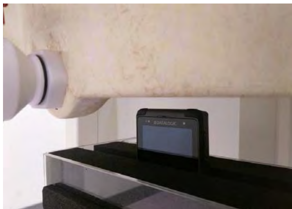
Fig.14 EUT Top side to flat phantom
