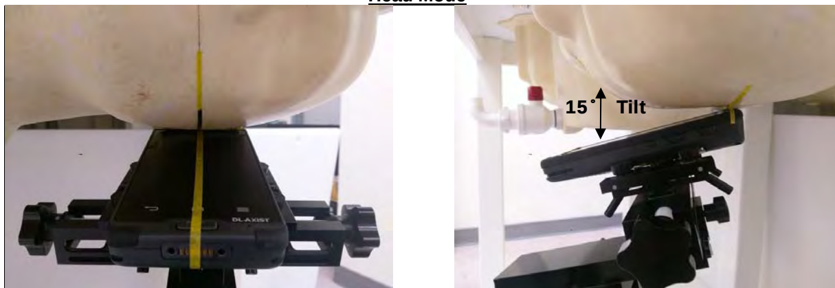
Fig.6 Left Head Section / Ear-Tilt Position(15°)
