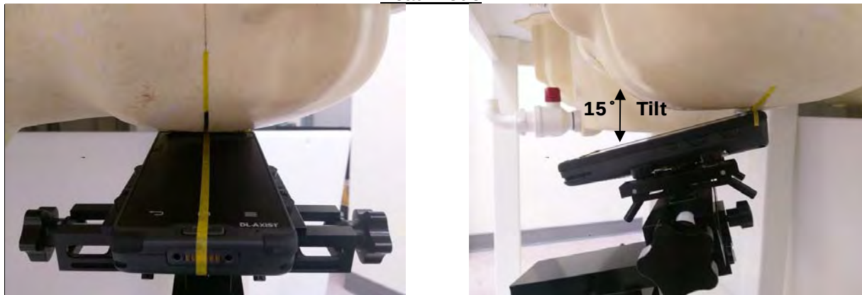
Fig.6 Left Head Section / Ear-Tilt Position(15°)
