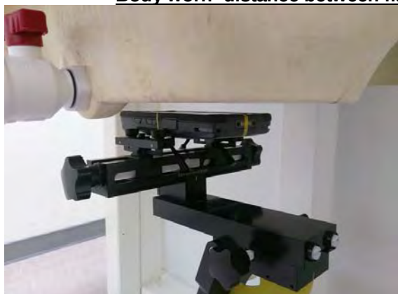
Fig.7 EUT Front side to flat phantom
