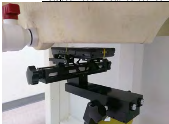
Fig.9 EUT Front side to flat phantom
