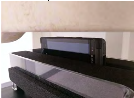
Fig.12 EUT Left side to flat phantom
