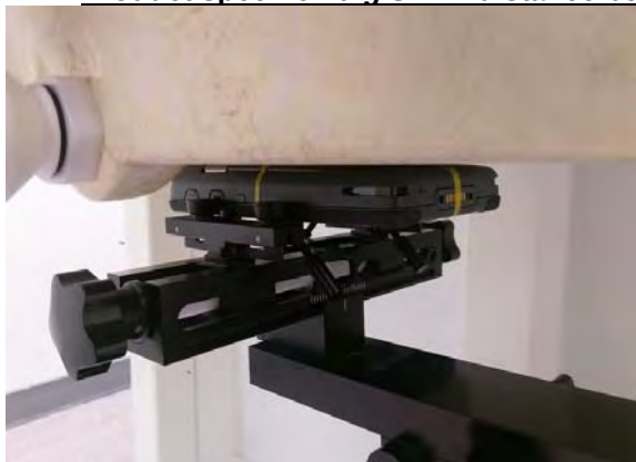
Fig.15 EUT Back side to flat phantom
