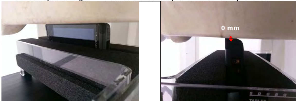
Fig.18 EUT Left side to flat phantom
