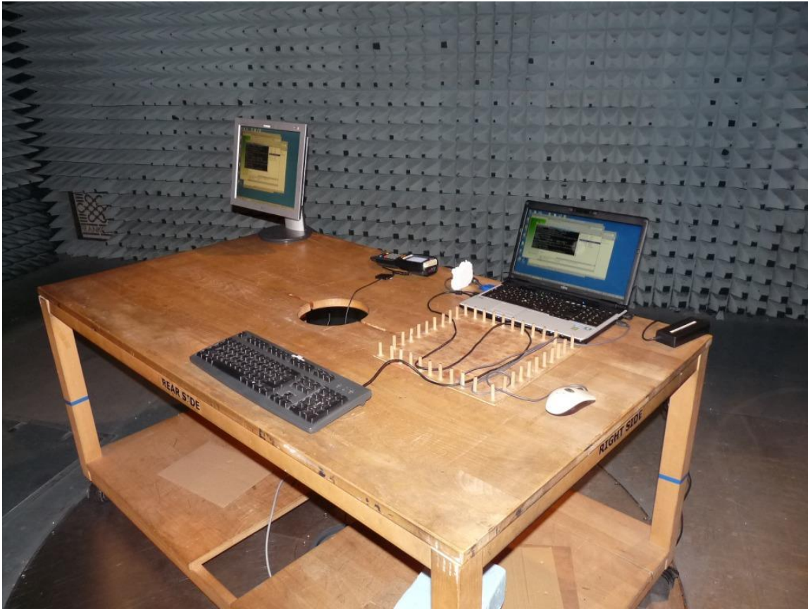
Photo 7: Test setup for radiated measurements (unintentional radiator §15), front view, Setup AF01
