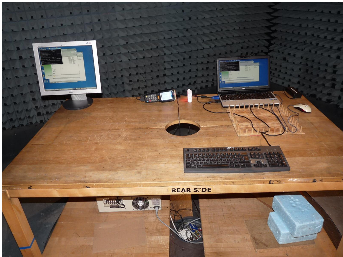
Photo 1: Test setup for radiated measurements (unintentional radiator §15)
