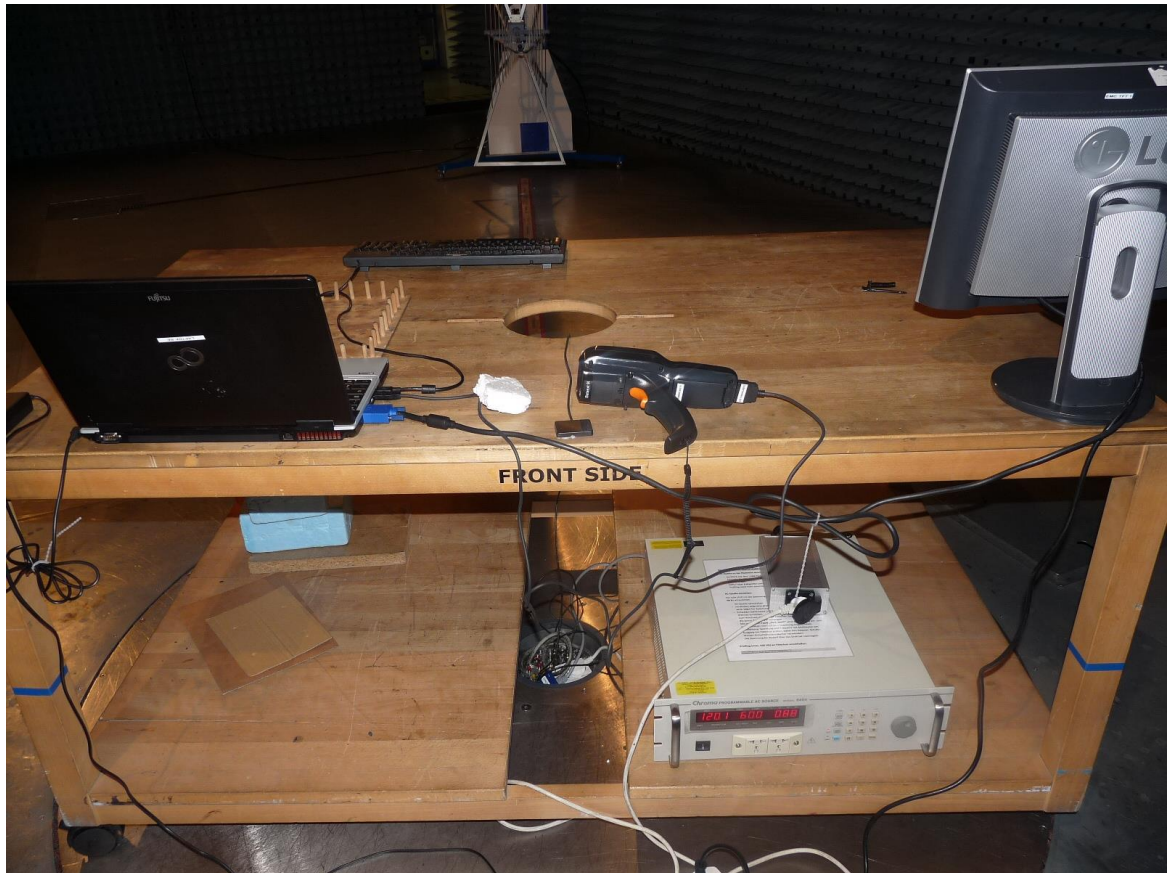
Photo 2: Test setup for radiated measurements (unintentional radiator §15)
