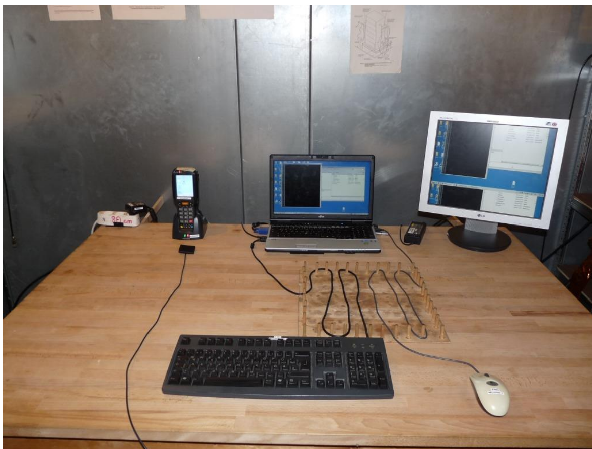
Photo 1: Test setup for conducted measurements (AC Port (power line), unintentional radiator §15)
