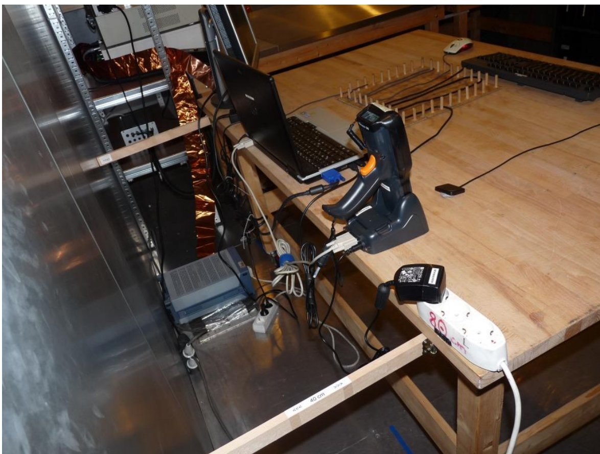
Photo 2: Test setup for conducted measurements (AC Port (power line), unintentional radiator §15)
