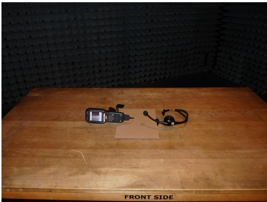
Photo 3: Test setup for radiated measurements (unintentional radiator §15); Setup AJ01
