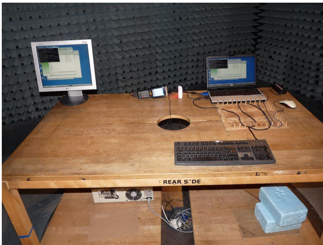
Photo 1: Test setup for radiated measurements (unintentional radiator §15); Setup AH01
