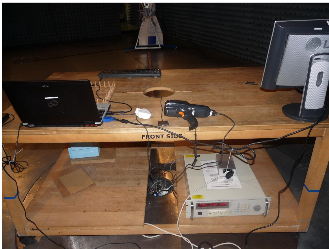
Photo 2: Test setup for radiated measurements (unintentional radiator §15) ; Setup AH01
