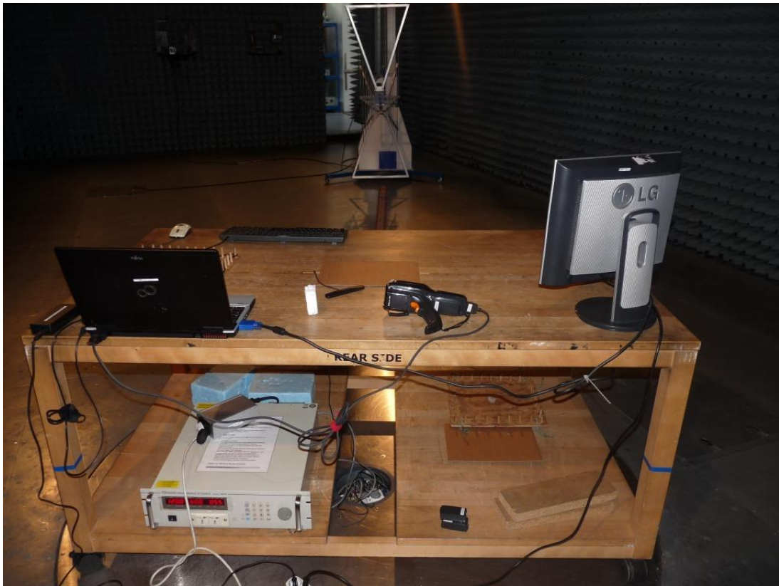
Photo 2: Test setup for radiated measurements (unintentional radiator §15)
