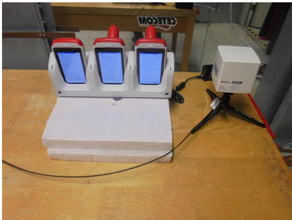
Photograph 4: Measurements in the anechoic chamber, 10cm distance between measurement probe and EUT
