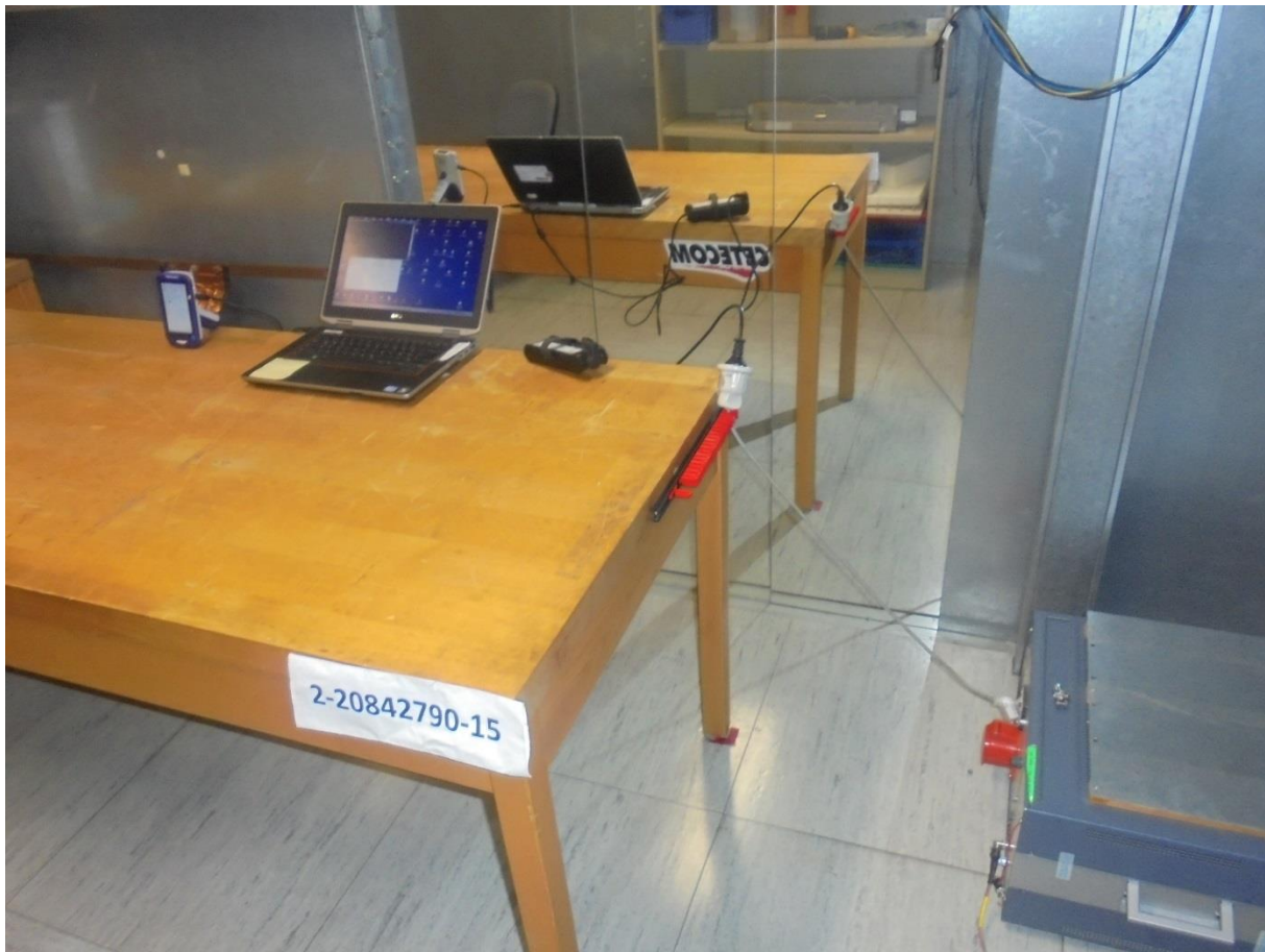
Photograph 1: AC-Power Line Conducted Emissions set-up (overview_front side)
