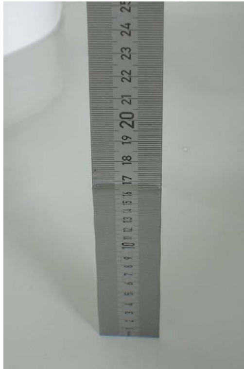
Fig. 12: Liquid depth for 2450 MHz body worn measurements.
