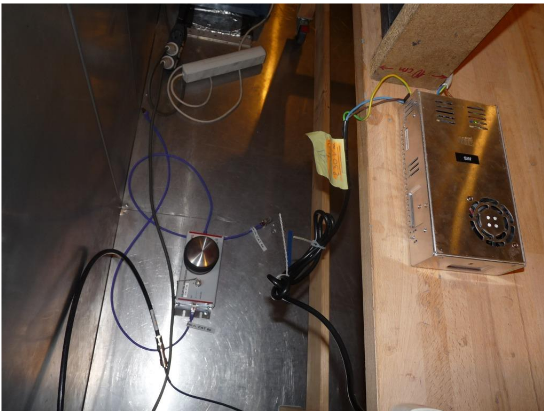
Photo 2: Test setup for conducted measurements, unintentional radiator (§15) 3-slot-cradle setup.
