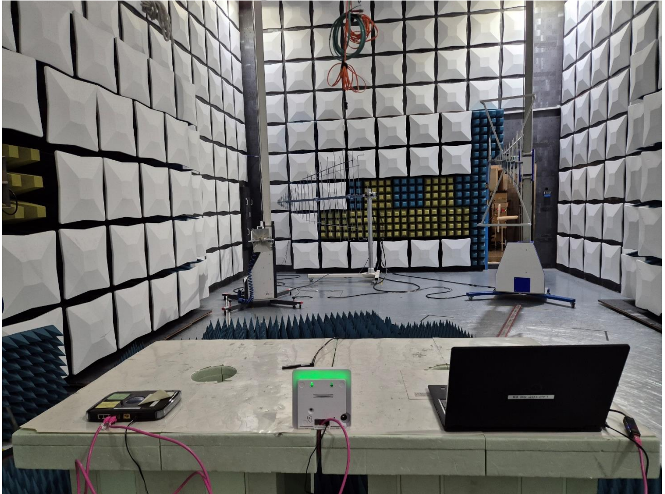
Photo 3: Test setup for radiated measurements, unintentional radiator (semi-anechoic chamber 1 GHz – 18 GHz)
