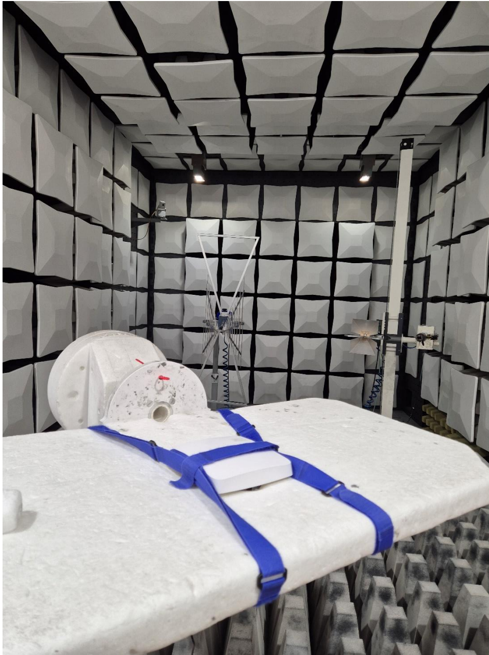
Photo 6: Test setup for radiated measurements, intentional radiator (fully anechoic chamber, above 1 GHz – 24 GHz;
