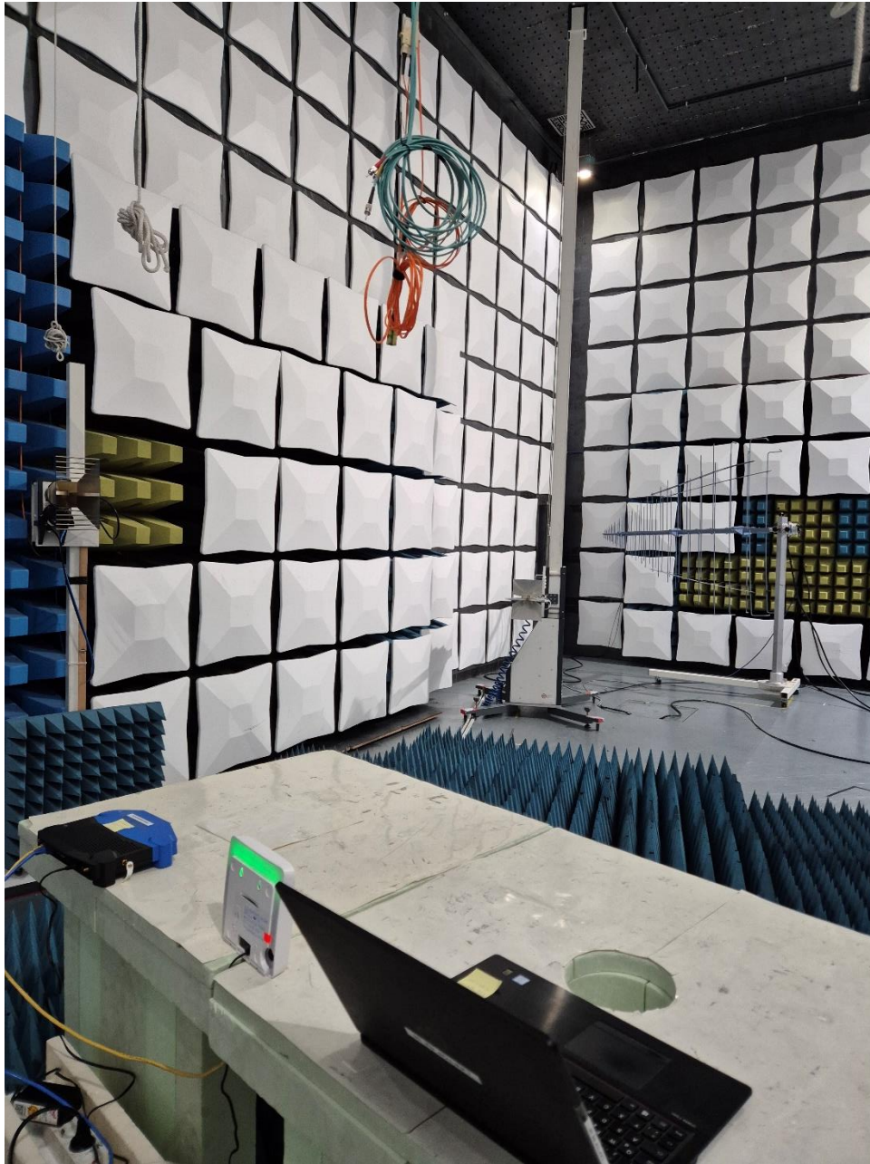
Photo 3: Test setup for radiated measurements, unintentional radiator (semi-anechoic chamber 1 GHz – 18 GHz)
