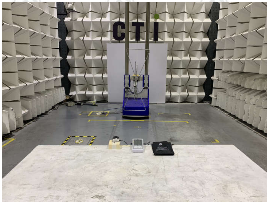
Radiated spurious emission Test Setup-1(Below 1GHz)
