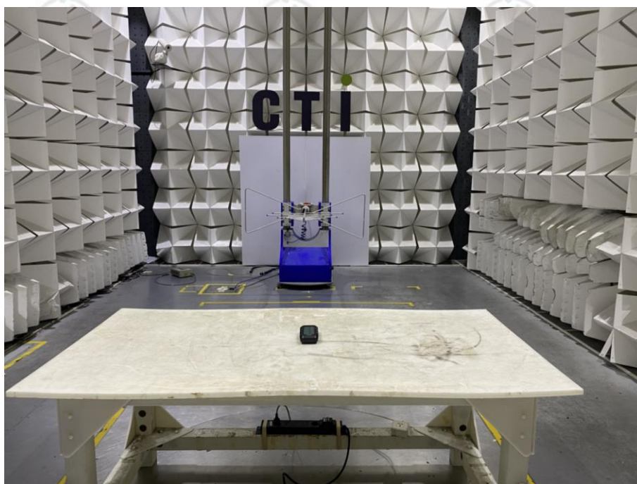
Radiated spurious emission Test Setup-1(Below 1GHz)
