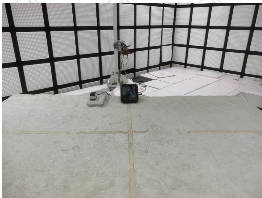
Radiated spurious emission Test Setup-2(Above 1GHz)
