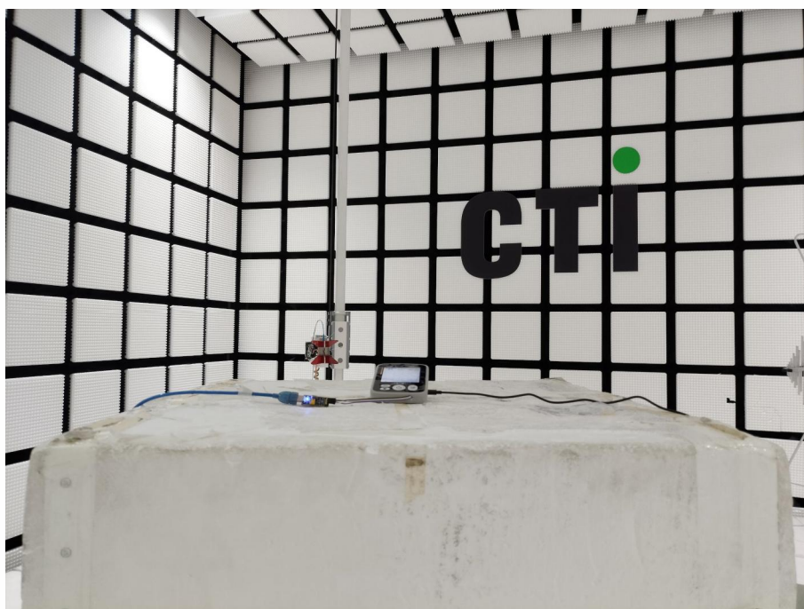
Radiated spurious emission Test Setup-2(Above 1GHz)
