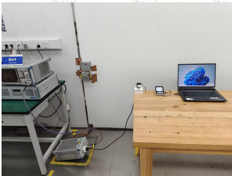
Conducted Emissions Test Setup
