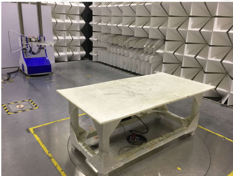
Radiated spurious emission Test Setup-2(30MHz-1GHz)
