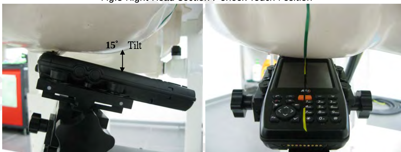
Fig.4 Right Head Section / Ear-Tilt Position(15°)
