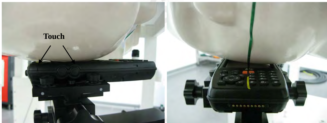
Fig.3 Right Head Section / Cheek-Touch Position
