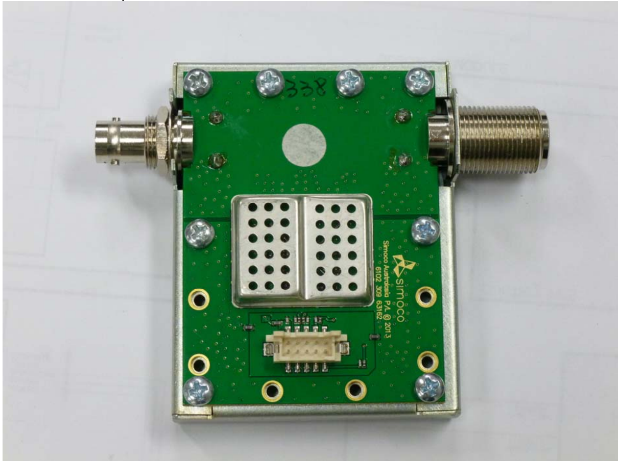
VSWR detector top with shields
