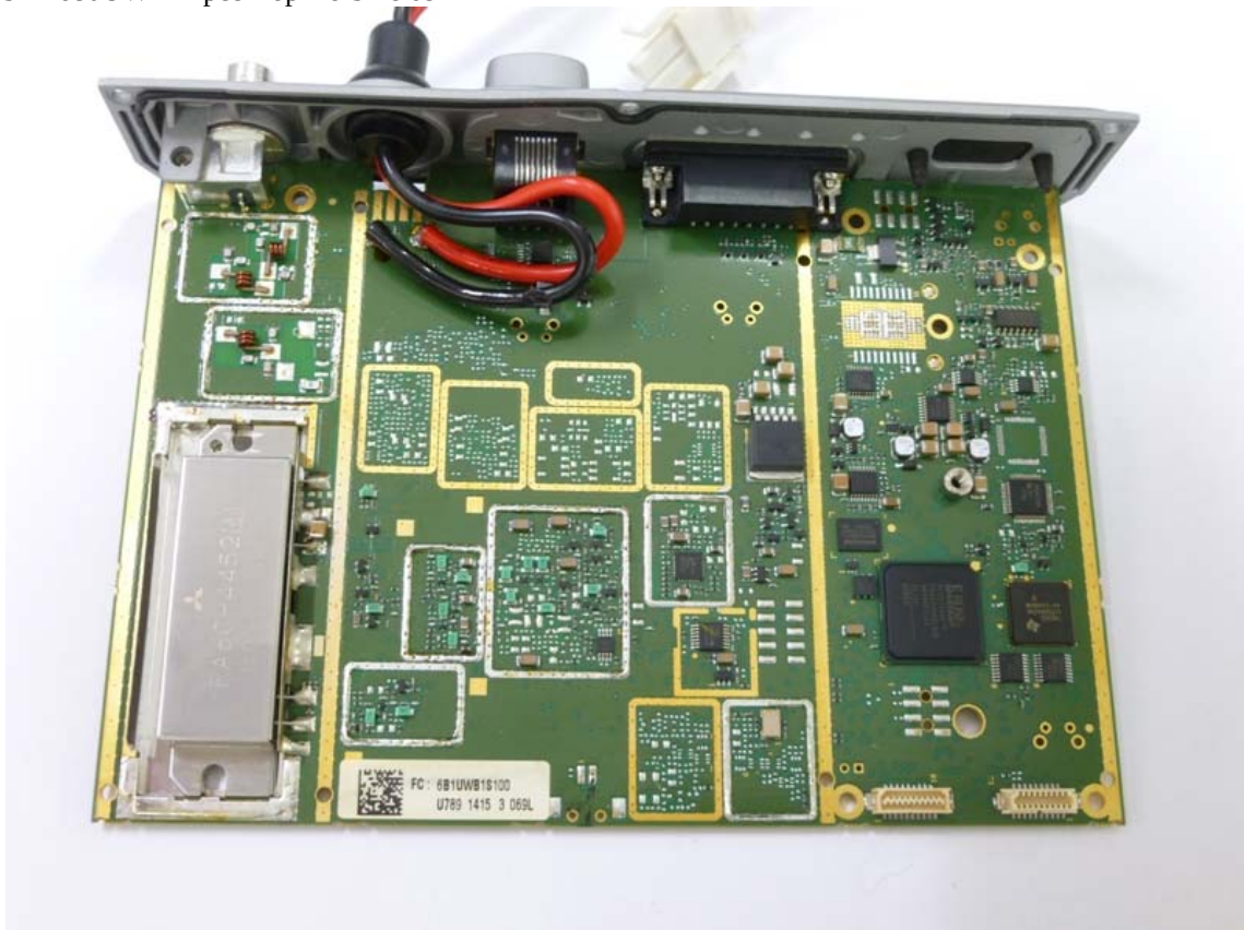
SDB680UW TX pcb Top No Shields
