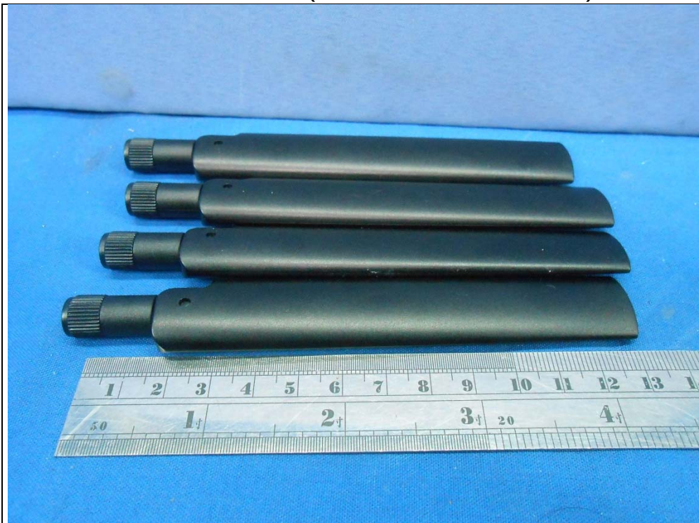
WWAN Antenna (Model: 98619ZSAX025)
