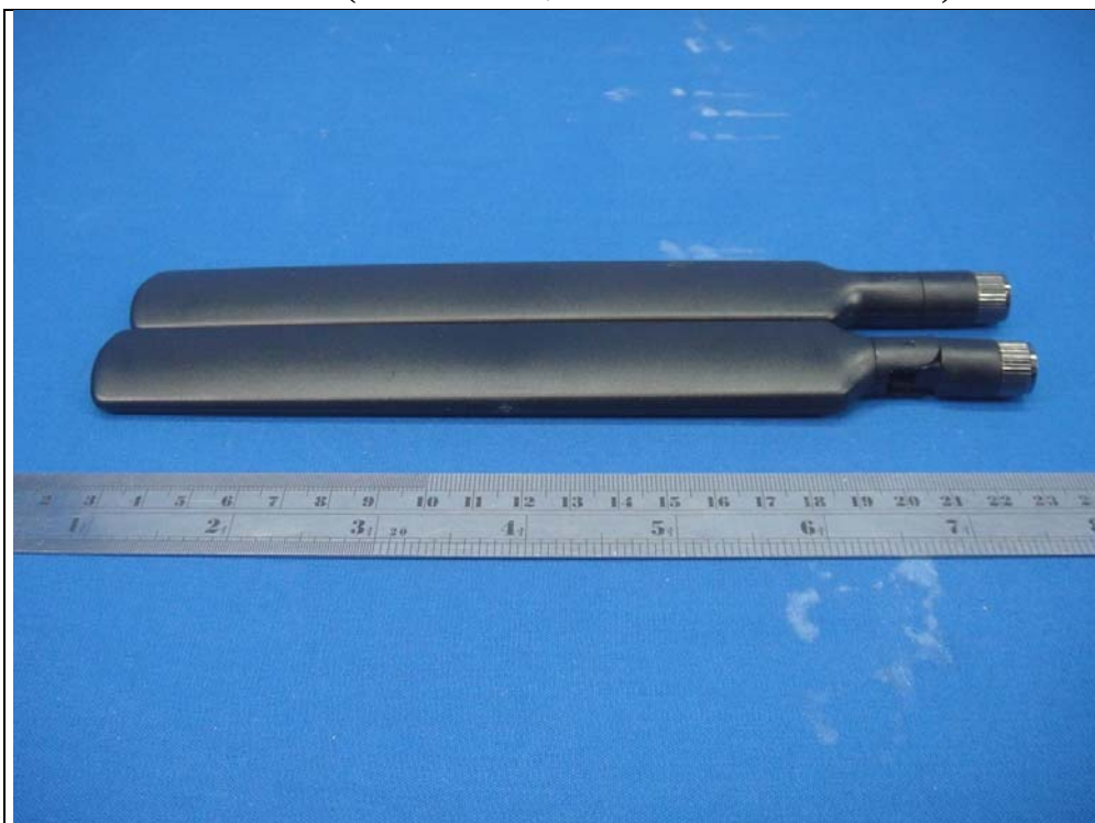
LTE antenna (Brand : Pulse, Model : SPDA24700/2700)
