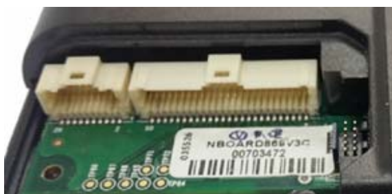
Figure 9: SmartHub Underdash OBC Interface connectors
