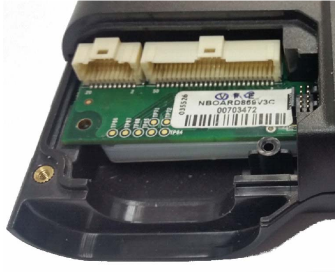
Figure 8: SmartHub Underdash OBC Interface connectors
