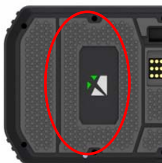
Picture 6: Tablet NFC Proximity Reader Area
