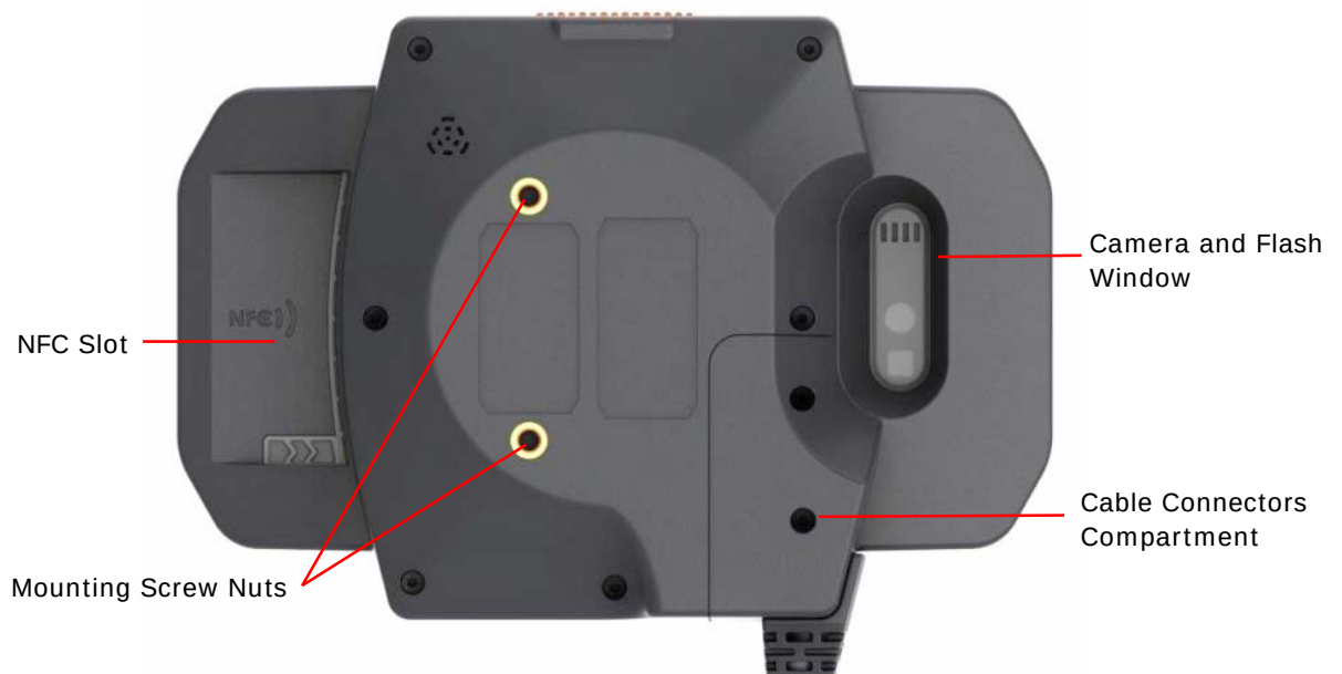
Figure 9: Cradle Rear View Components
