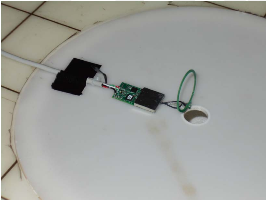
8616103 module with 8001204 antenna
