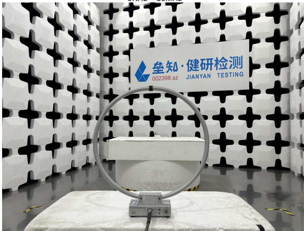
Radiated Spurious Emission 9KHz ~ 30MHz
