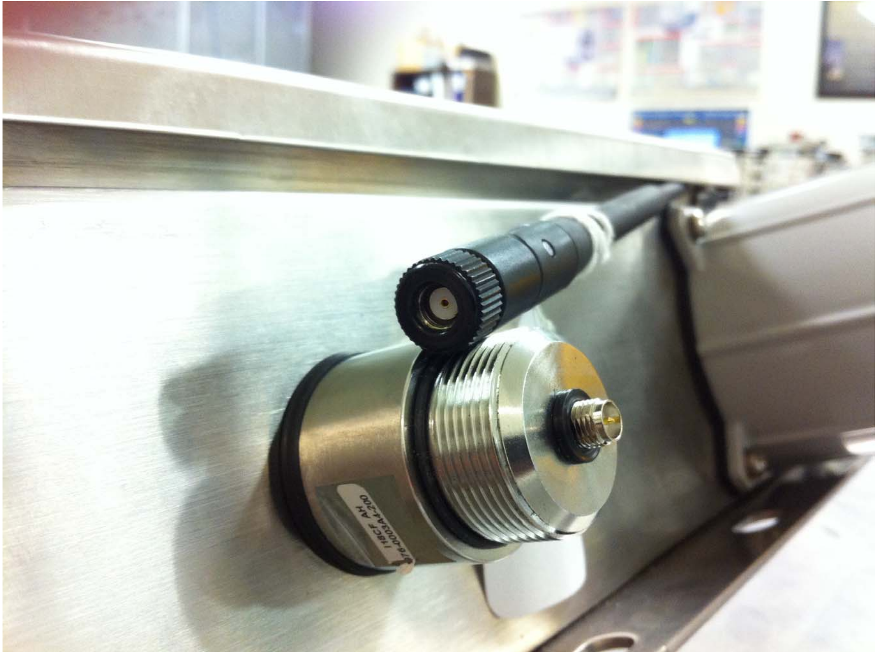
Close-up View of Antenna Connectors – Note Polarity of Center Pin is Reversed
