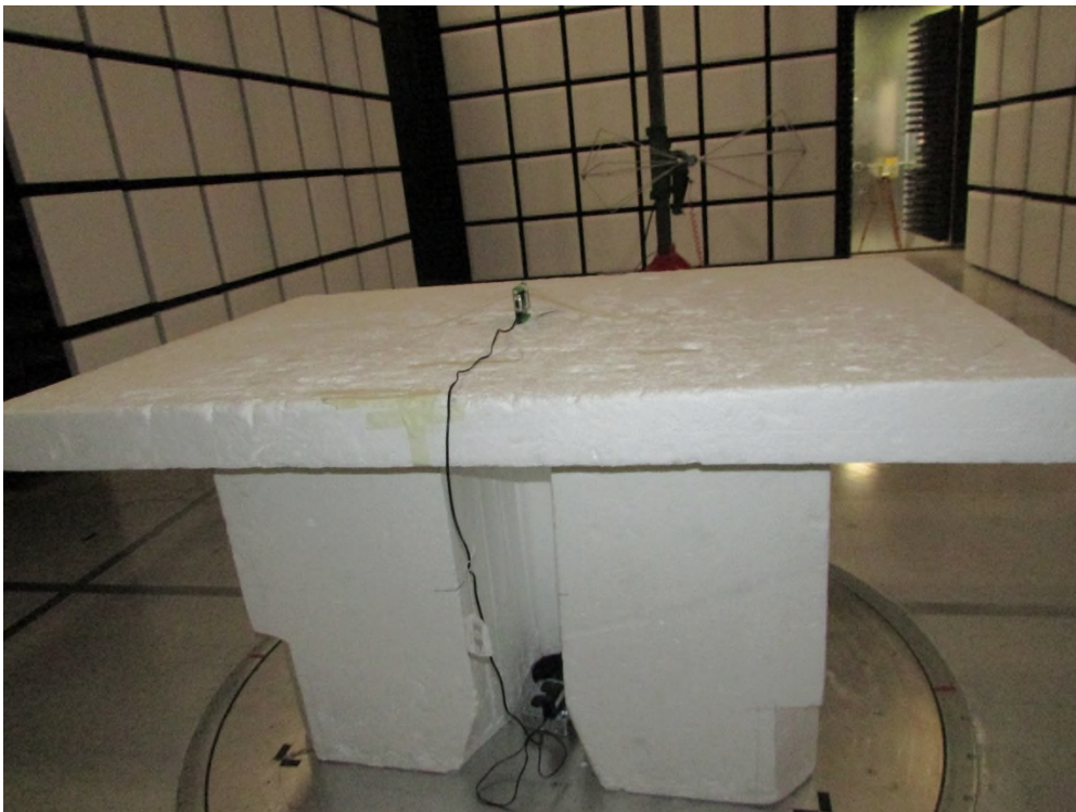
Figure 2: Radiated Emissions – Back – Y-Plane – Below 1GHz
