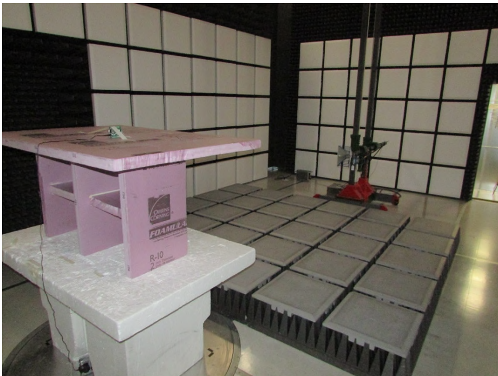
Figure 4: Radiated Emissions –Back – Y-Plane – Above 1GHz
