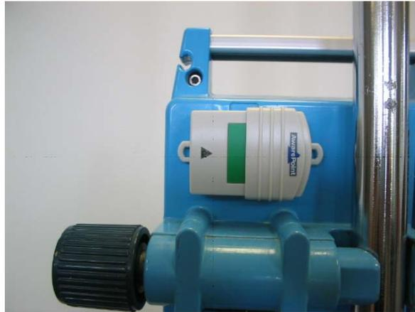
Figure 64 - Tag Double-Sided Tape Attachment
