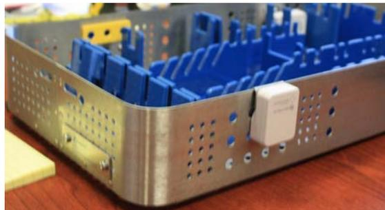
Figure 69 - Autoclave Tag on Outside of Tray
