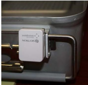
Figure 70 - Autoclave Tag in Bracket
