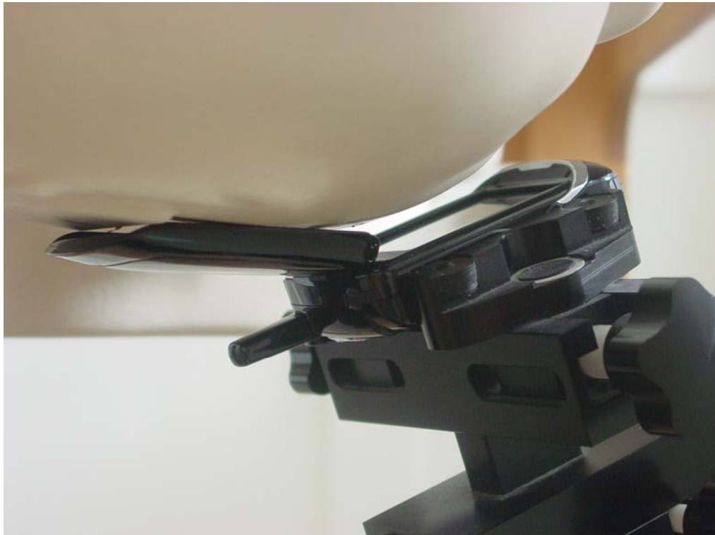
Picture B6: Right Hand Touch Cheek Position
