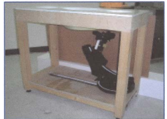
Picture6: Generic Twin Phantom
