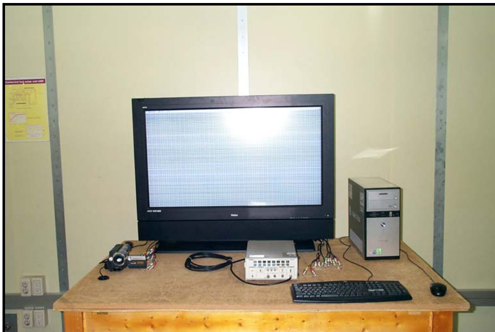
Photograph 1: Setup for Conducted Emissions <Digital Mode>
