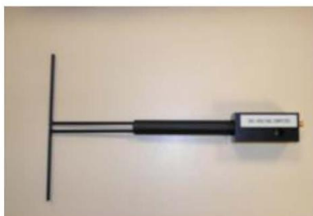
Figure 1 – Satimo COMOSAR Validation Dipole
