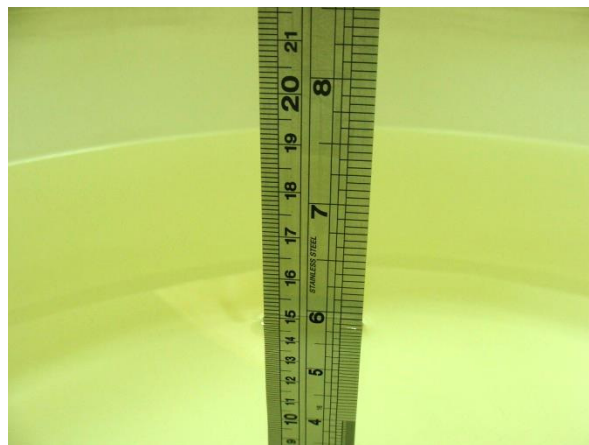
Fig 10.2 Photo of Liquid Height for Body SAR
