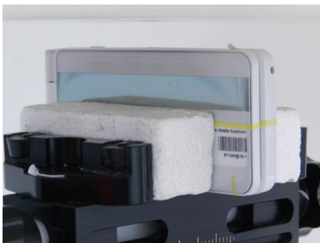
Right Side, Test Separation 10 mm
