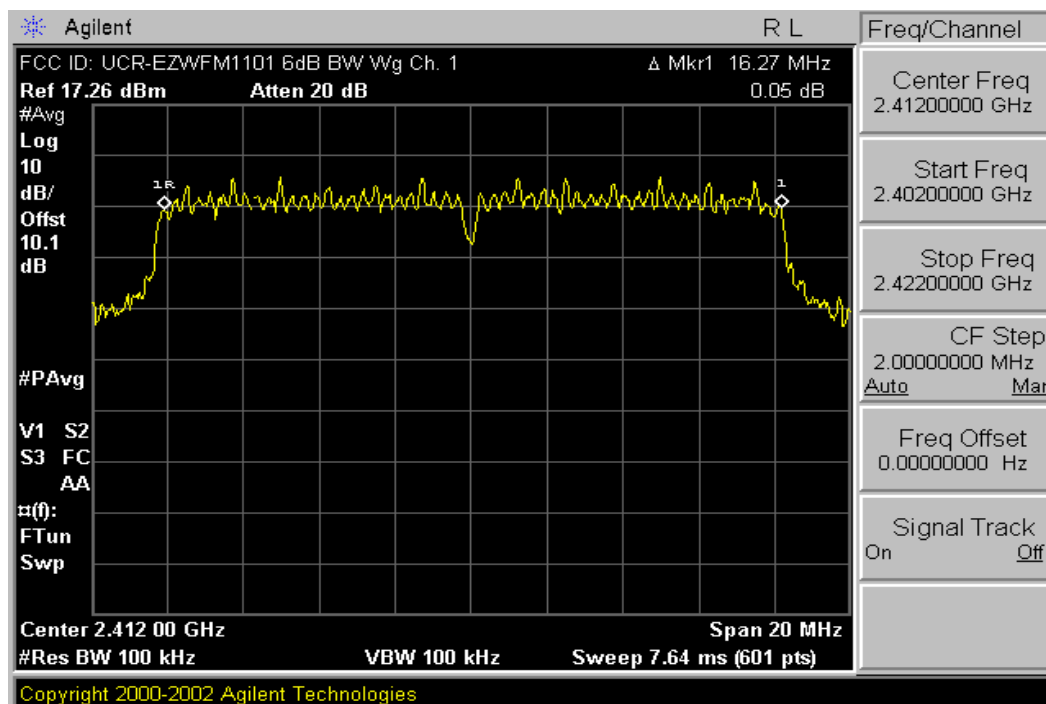
Plot 6-4. 6dB Bandwidth Plot (802.11g – Ch. 1)
