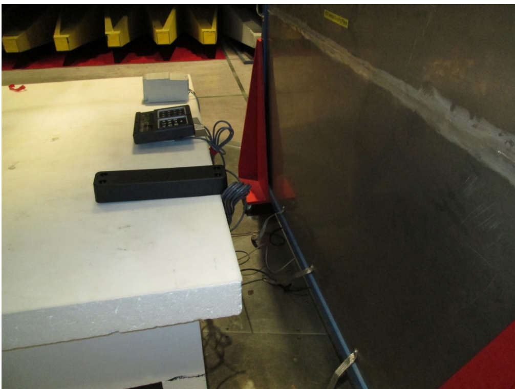
Photo 4.3.2 Test setup regarding measurement of radio frequency voltage on mains.
