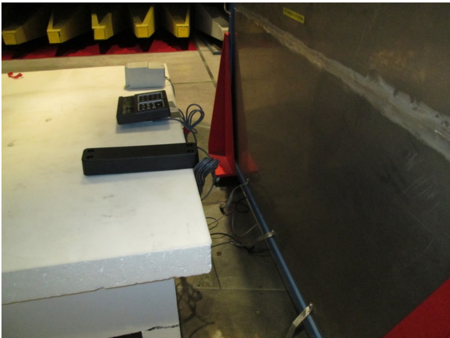
Photo 2.1.2 Test setup regarding measurement of radio frequency voltage on mains.
