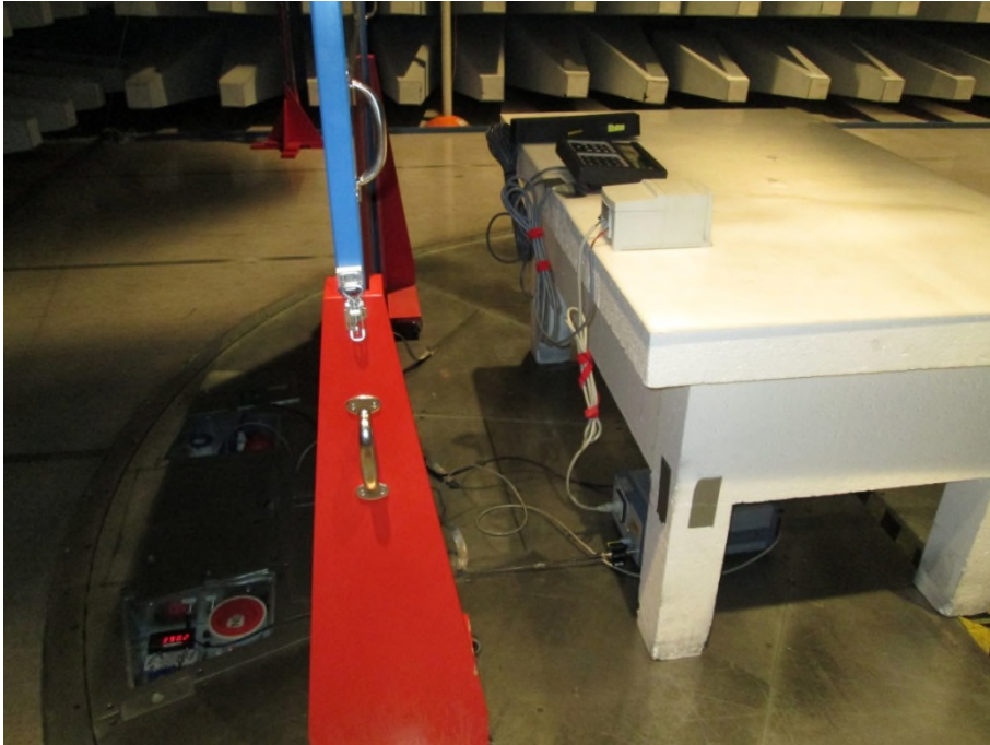
Photo 2.1.1 Test setup regarding measurement of radio frequency voltage on mains.
