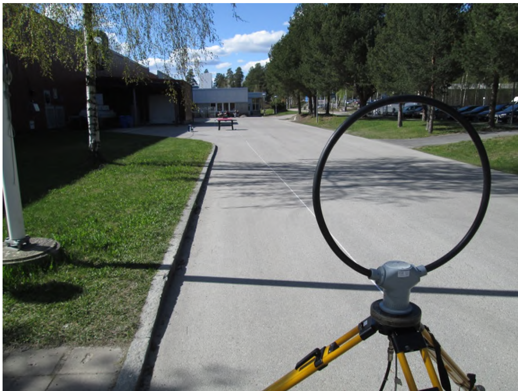
Photo 2.2.3 Test setup regarding measurement of radio frequency electromagnetic field. Verification measurement outdoors. 30 m measurement distance.
