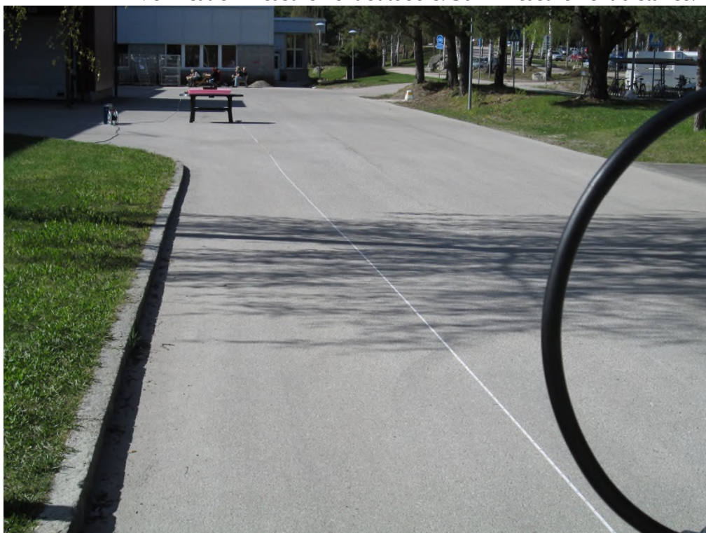
Photo 2.2.4 Test setup regarding measurement of radio frequency electromagnetic field. Verification measurement outdoors. 30 m measurement distance.
