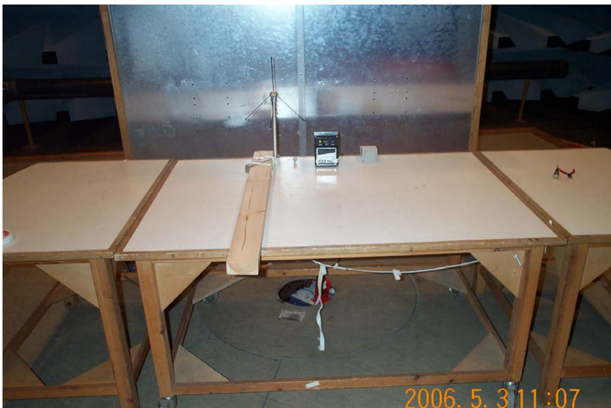
Photo A2.4 Test setup for conducted emission.
