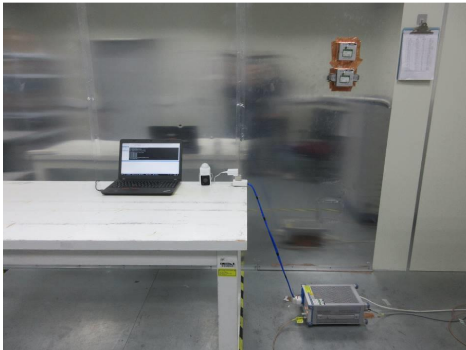
POWERLINE CONDUCTED EMISSIONS MEASUREMENT SETUP
