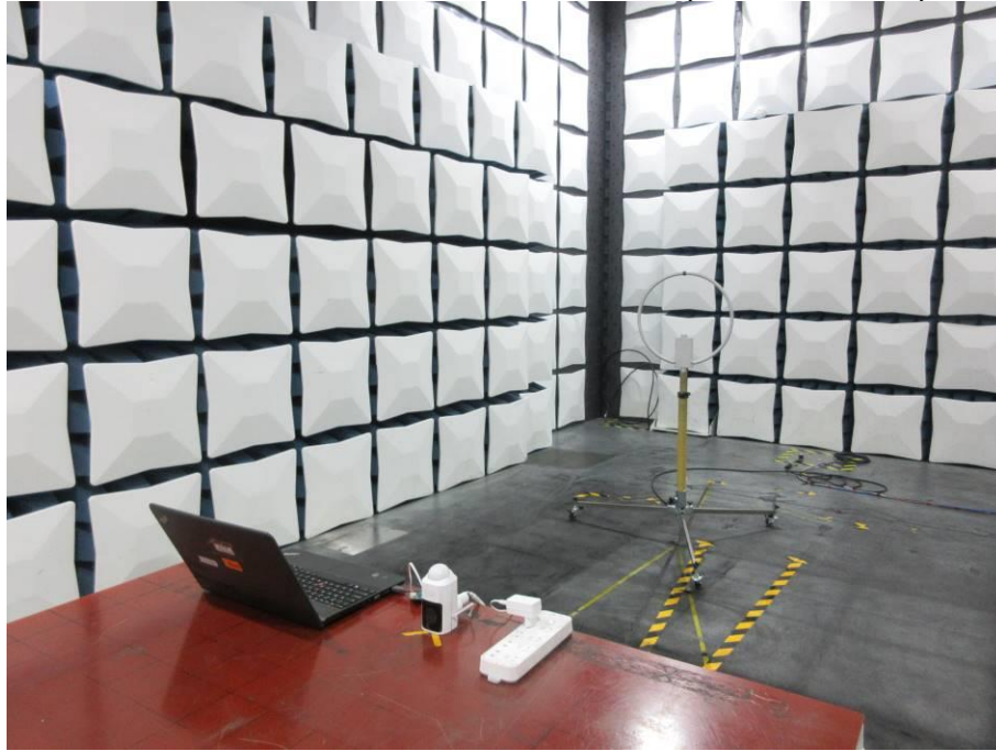
RADIATED RF MEASUREMENT SETUP (9KHz ~ 30 MHz)
