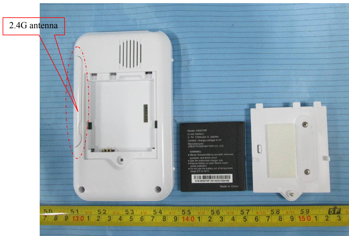
EUT-Battery off View
