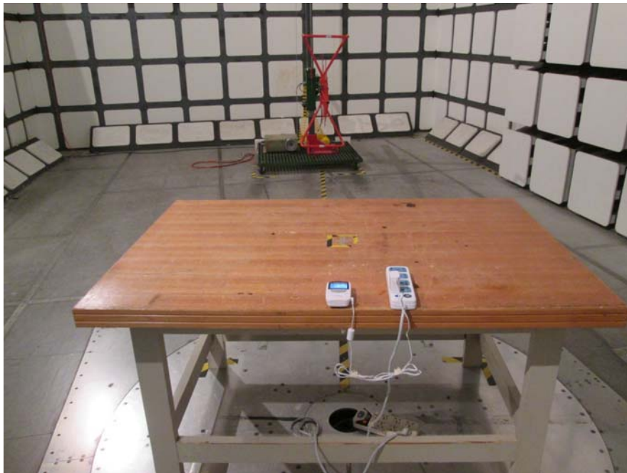
Radiated Emissions - Rear View (Below 1 GHz, Charging by KINGS adapter))
