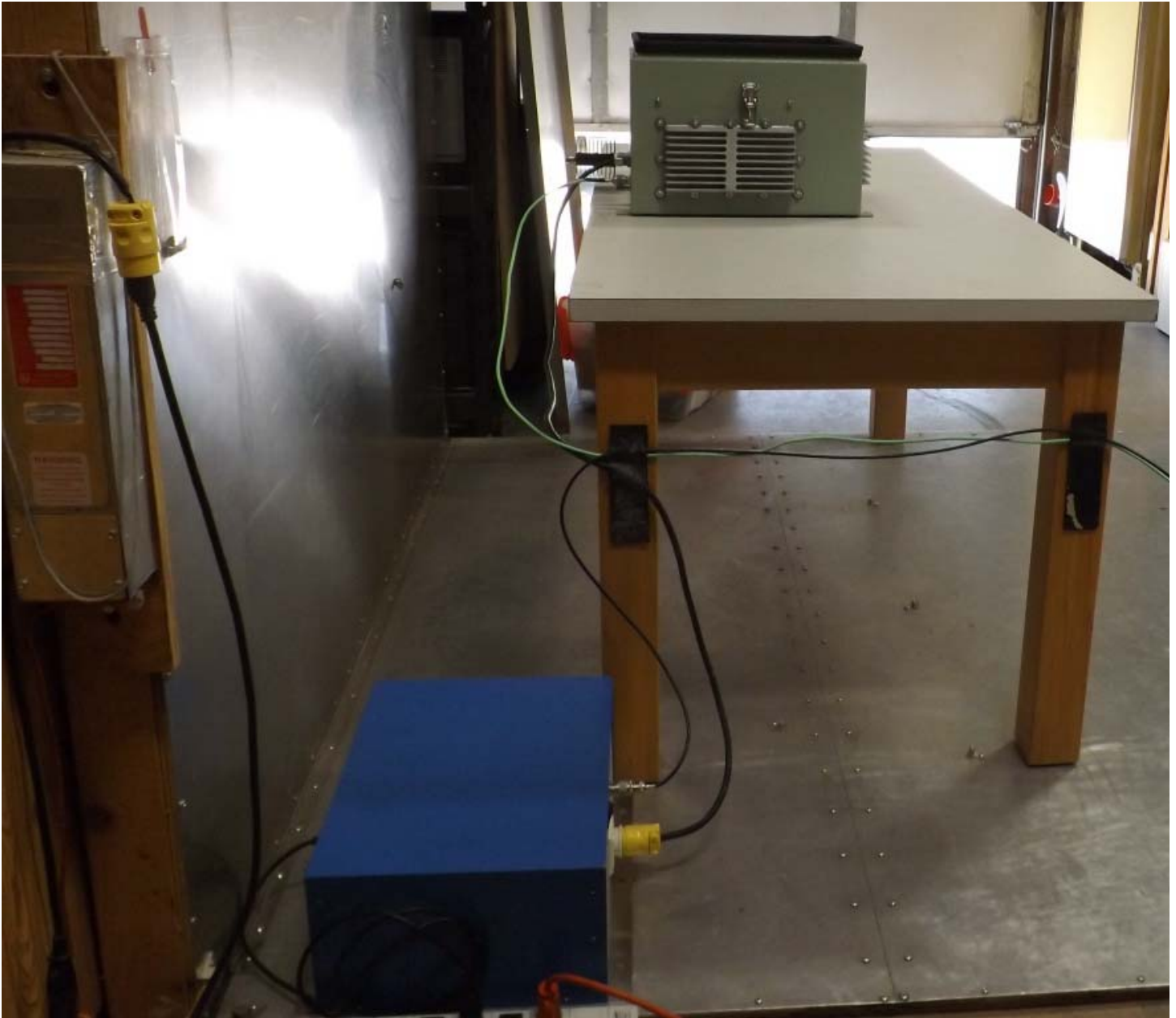
Figure E24.4 – Setup – Power Line Conducted Measurements
