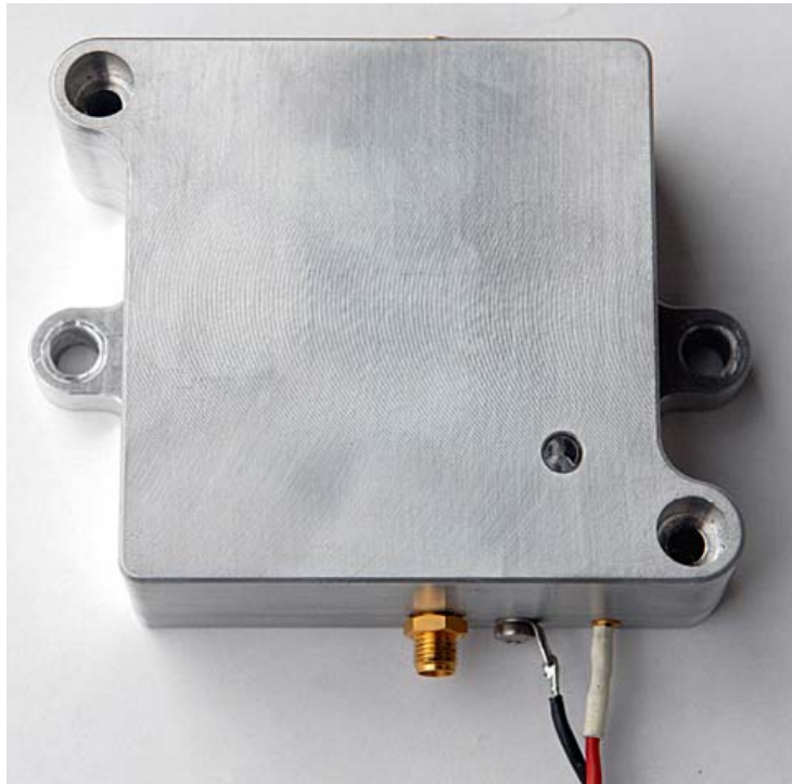
Power amplifier enclosure
