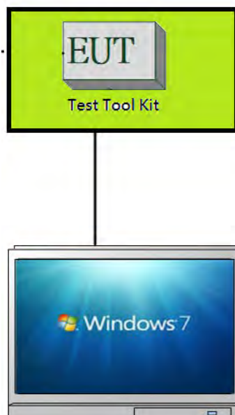
Fig. 2-1 Configuration of Conducted and Radiated Tested System
