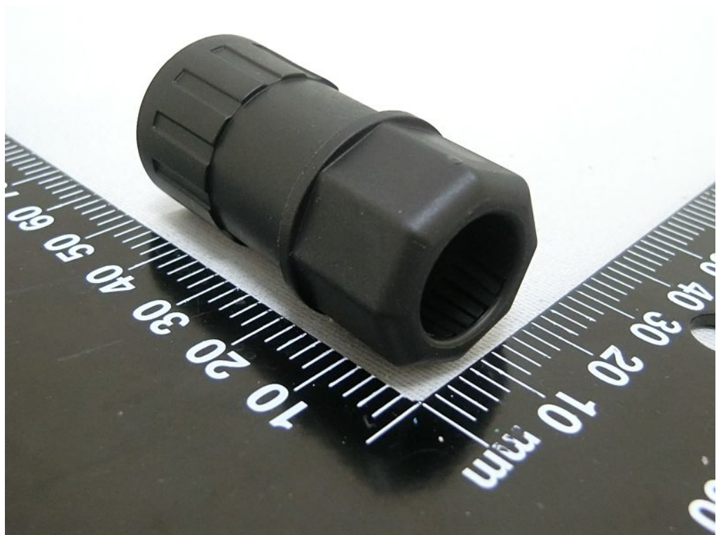
Waterproof Covering (Cable Gland) 2 used for EUT 2
