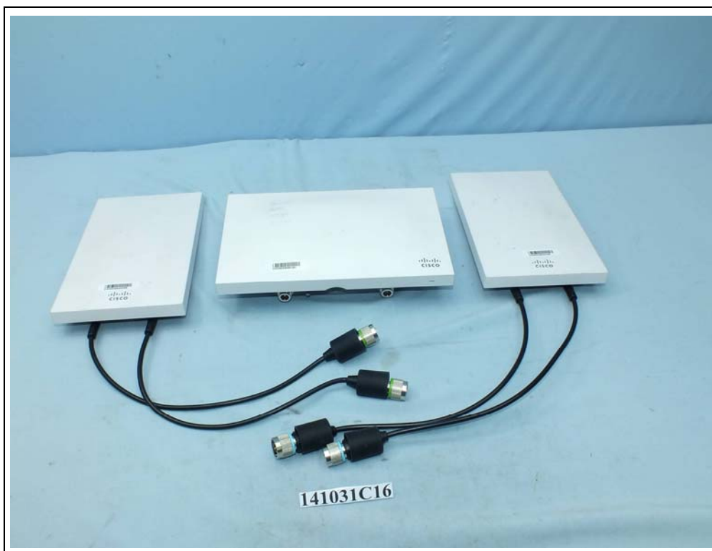
EUT with sector antenna
