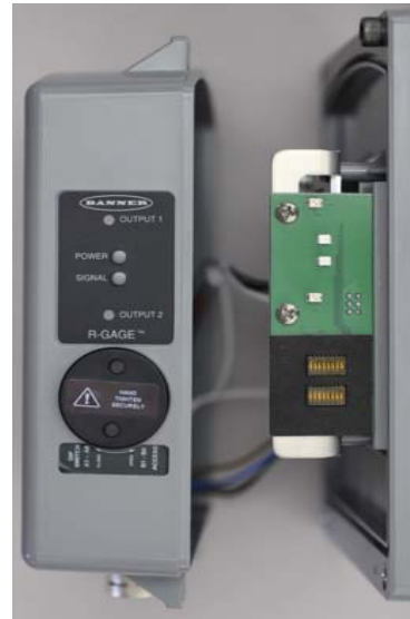
Figure 14, Assembly Side View
