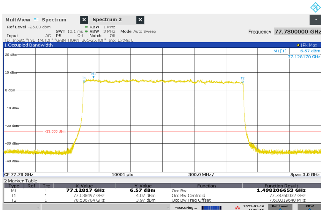
Plot 2: Power spectral density tested under extreme condition TmaxVnom
