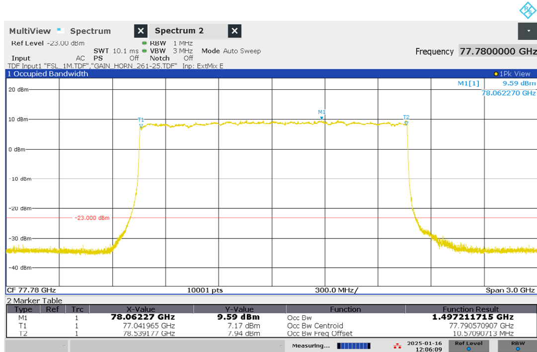
Plot 1: Power spectral density tested under nominal condition TnomVnom
