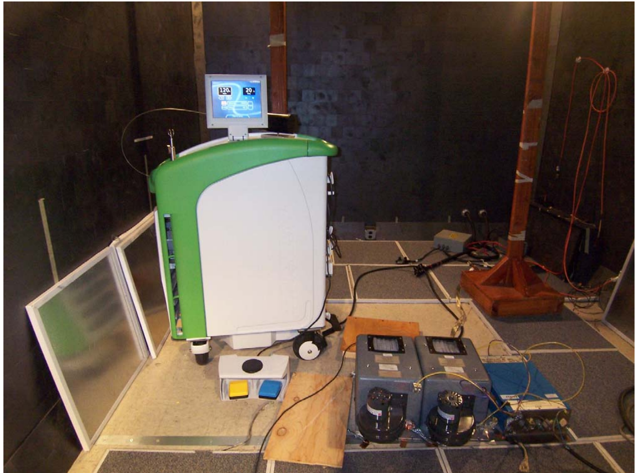
Photograph 1. Conducted Emissions Test Setup
